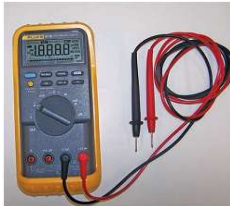
Figure1- 9 Typical multifunctional, low-impedance multimeter.
