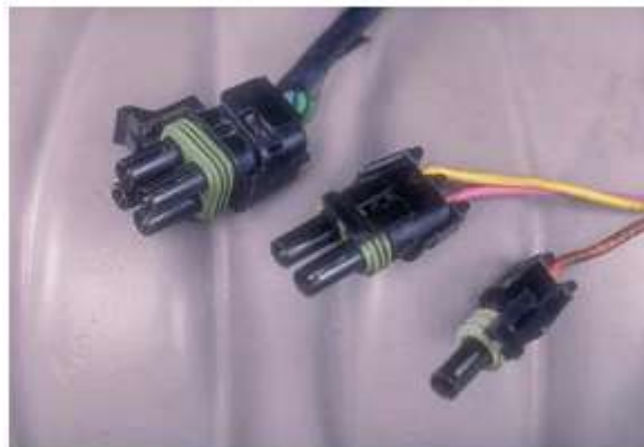
Figure1- 20 Weather-pack connector is used to prevent connector corrosion
