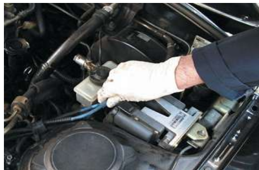
Figure1- 3 Protective gloves such as these vinyl gloves are available in several sizes. Select the size that allows the gloves to fit snugly. Vinyl gloves last a long time and often can be worn all day to help protect your hands from dirt and possible hazardous materials.
