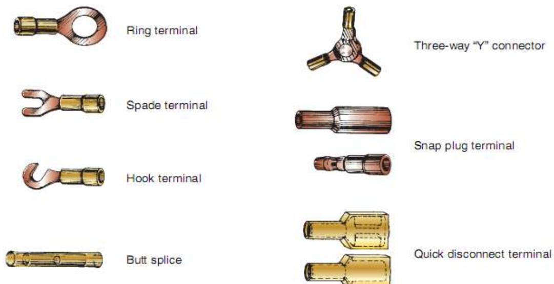
Figure1- 16 Examples of primary wire terminals and connectors used in automotive applications.
