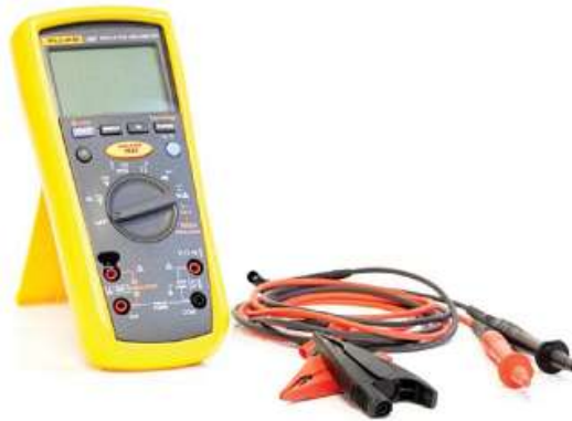
Figure1- 10 An insulation meter is used on many HEVs to determine insulation leaks in the high-voltage system.
