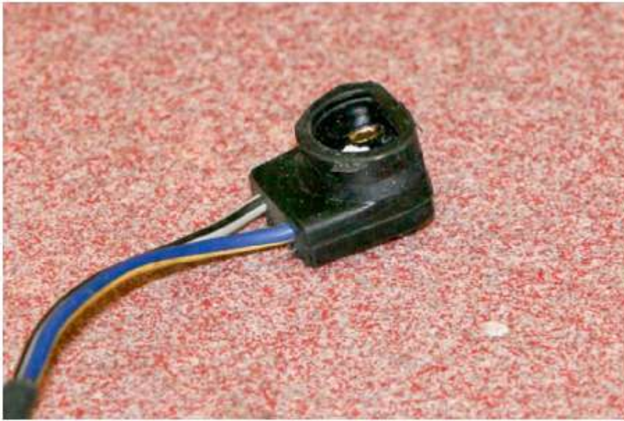
Figure1- 17 Molded connectors cannot be disassembled to replace damaged terminals or to test.
