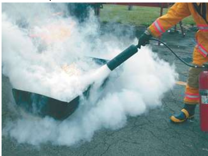
Figure1- 6 A CO 2 fire extinguisher being used on a fire set in an open steel drum during a demonstration at a fire department training center.
